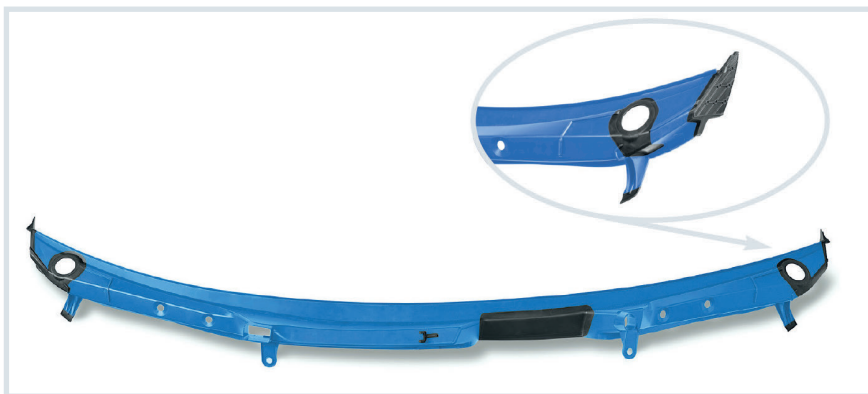
Fig. 2. The molded part is made of two thermoplastic components, specifically the main body made of polypropylene, which is combined with elastic TPE-sections at the contact points with the car body and in the passage areas for the windshield wipers. © Eldisy
