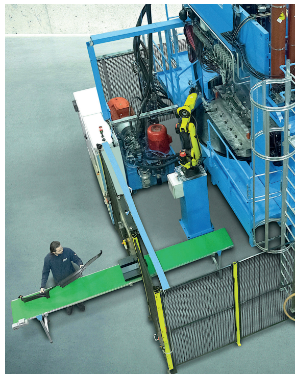
Fig. 5. Detailed view of the robot position for the molded part manipulation. © LWB-Steinl
